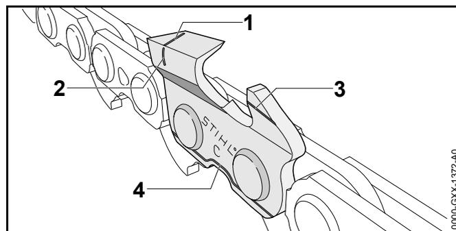
STIHL chain is manufactured with wear marks to help the operator identify excessive wear. The wear marks depicted above (1 - 4) must remain visible.
