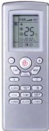
9. Use X-FAN button to turn on and off extended fan operation feature in cooling and DRY modes.
