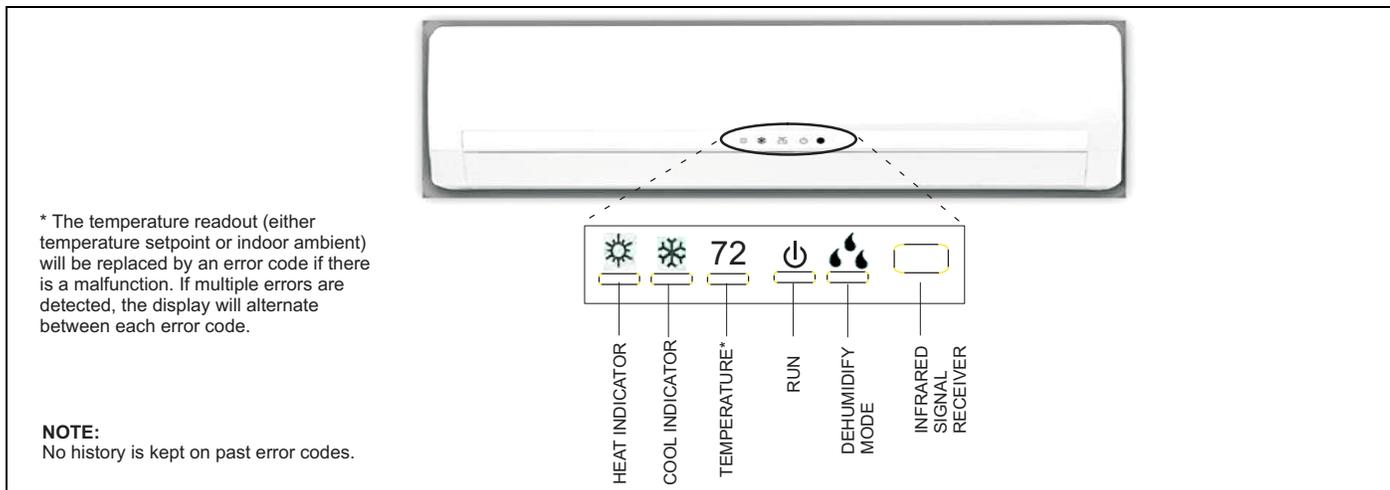
**FIGURE 4:** Indoor Unit Front Panel Indicators
