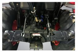
Telescopic Lower Links & Stabilizers Standard telescopic lower link ends and stabilizers allow the operator to easily connect & adjust a wide variety of 3-point implements.
