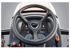
**Power Steering with Tilt** The standard power steering minimizes the effort required to make tight, repetitive turns. The steering wheel tilts to adjust for operator needs.
