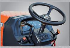
**Power & Tilt Steering** The standard power steering minimizes the effort required to make tight, repetitive turns. The steering wheel tilts with a compression style lever, allowing easy adjustment to fit operator
