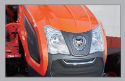
**Center Marker** The center ridge marker on the hood assists with maintaining straight lines during operation.
