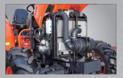
**Eco-Friendly Diesel Engine** The Common Rail Diesel Engine (CRDI) improves fuel efficiency while reducing noise levels. With this eco-friendly Stage 5 engine, the DK10 Series offers the operator a quiet work environment with powerful performance.
