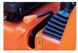
**4WD Engagement** The 4WD comes standard on all models and is engaged with an easy access lever.
