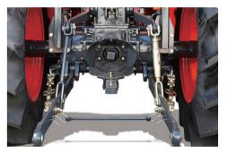
**Improved Performance** The large capacity hydraulic pump (14.5 gpm) combined with high lift capacity (2,716 lbs.) increases productivity.
