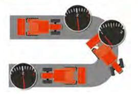
**Turn Assist Control** The optional Turn Assist Control kit will drop the engine rpm by 10% automatically when turning sharply. This feature allows for more precise work and reduces fuel consumption during sharp turns.
