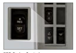
**PTO Cruise Control** With one touch, engine speed may be set to maintain steady PTO rpm to maximize working efficiency. When engaged, the operator may change the engine rpm by simply pressing a switch to increase or decrease the rpm.
