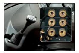
**Remote Hydraulic Valves and Joystick** Standard single lever joystick is valuable for loader operation or front implements. A standard single remote valve (2nd and 3rd optional) accommodate a wide variety of attachments and implements.
