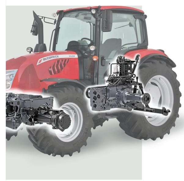
The **X6** standard series features an open-center hydraulic system with a total flow of 24.3gpm (92 lpm) allowing efficient operation of all hydraulic functions. A dedicated pump supplies 16.4 gpm (62lpm) to the rear remote valves and 3 point hitch, while a separate gear pump supplies 7.9gpm (30lpm) to the steering system ensuring smooth and precise turning in any conditions for enhanced operator comfort and productivity.
