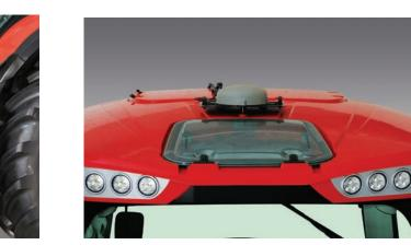
The automatic climate controls are conveniently built into a stylish roof console. An opening transparent roof hatch provides extra visibility for loader operations.
