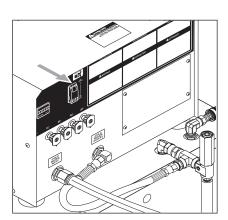
**STEP 5:** To stop machine, release the spray gun and machine will automatically stop in approximately 12 seconds. If machine is going to be unattended for long periods of time, turn water supply off and place switch in OFF position.
