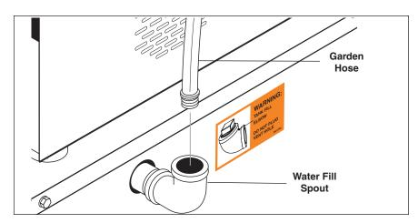
**STEP 4:** Do not turn power on to equipment until the heating module is filled with water, as severe damage may occur to heater elements.
