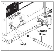
**STEP 2:** Connect water supply hose (garden hose) to inlet connector. Do not allow acid or abrasives to be pumped through system. Turn on water.
