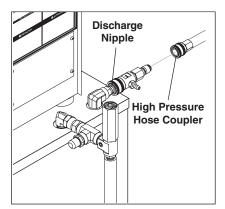
STEP 1: Connect the high pressure hose quick coupler to the discharge nipple by sliding the quick coupler collar back and inserting the quick coupler onto the discharge nipple and pushing the quick coupler collar forward to secure it. Secure desired pressure nozzle into variable pressure wand coupler.
