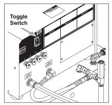
**STEP 1:** Rinse all lines (and injector) with clean water, to remove any soap residue then turn toggle switch off.
