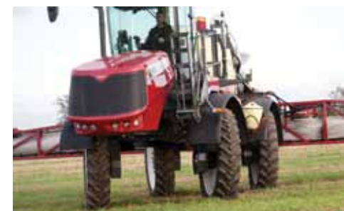
Crab steering - in difficult conditions and manoeuvring
