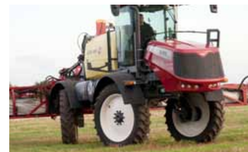
4-wheel steering - field mode
