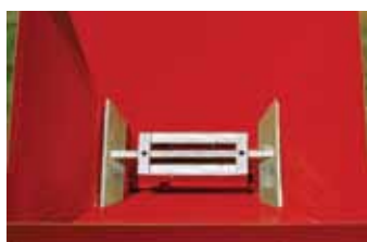
The optional magnet removes nails and metal debris from grain.
