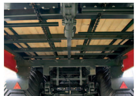
Chain-and-slat conveyor with split driveline and gearbox positioned in the middle.
