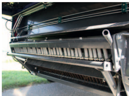
Each knife is spring protected against foreign obstacles. The knife will immediately return to working position once the obstacle has passed.
