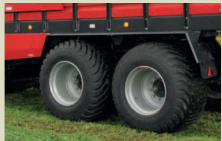
Large 600/55 - 22.5 tyres are standard fitted on Kverneland Taarup 10055.
