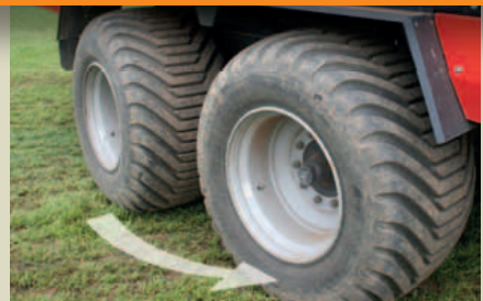
Actively steered wheels for improved maneuverability.
