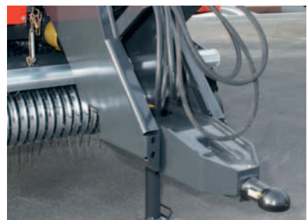
... or ball heads making it possible to choose the solution suiting your tractor.
