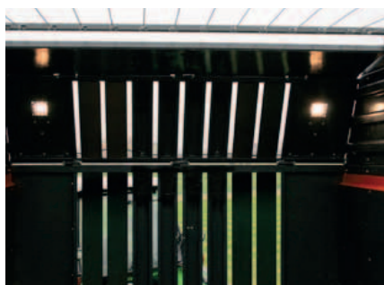
The deflector plates ensure optimum distribution of the crop throughout the entire chamber.
