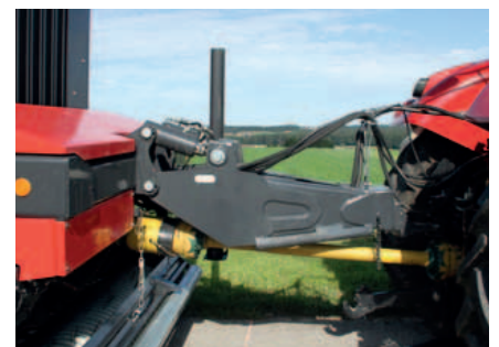
The Kverneland Taarup models are optional fitted with hydraulically articulated pin-hitch drawbar.
