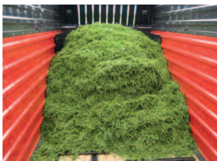
Strong and straight side walls ensure smooth transfer of crop to the rear of the chamber.
