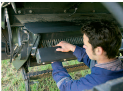
The knives are quickly released and changed without the use of tools.
