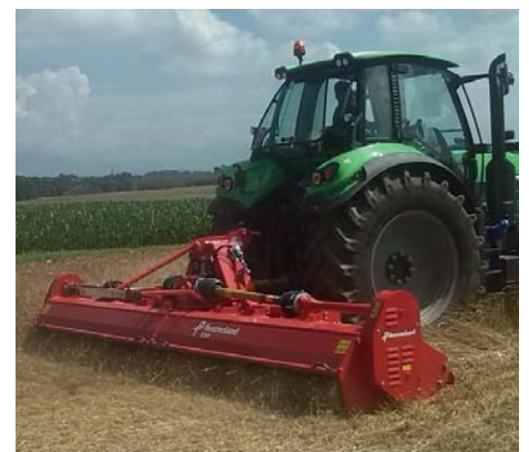
The central gearbox (250hp) is equipped with free wheels; the lateral transmission (5 belts each side) with an automatic belt tensioner ensures reliability and a low maintenance effort.
