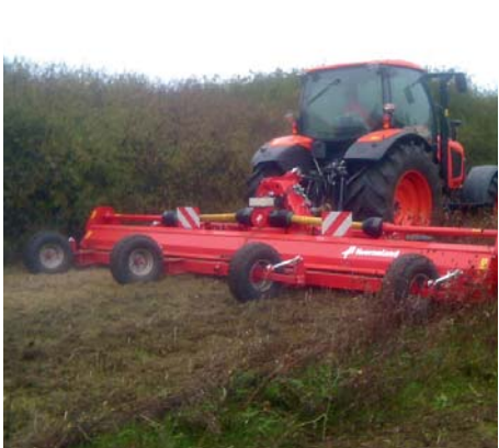
Semi pivoting wheels (10/8.0 x 12.8 ply) as option ensure a good stability and a constant working depth during field operations.
