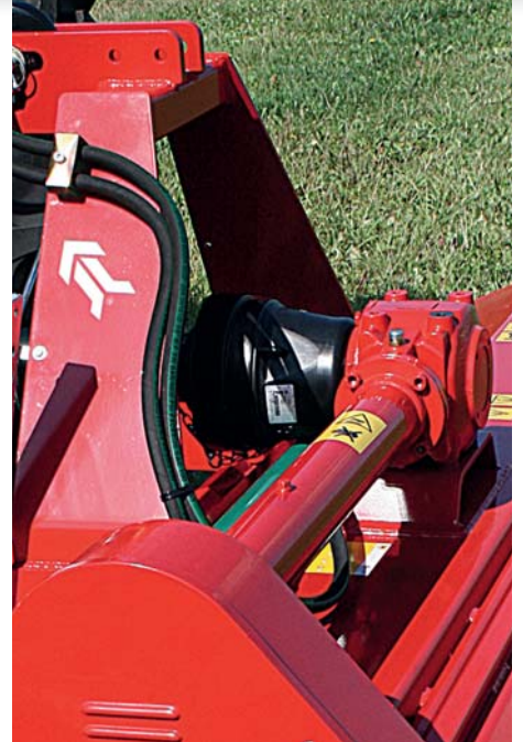
Gearbox up to 80hp - PTO speed drive 540 rpm. Protected by integrated free-wheel.
