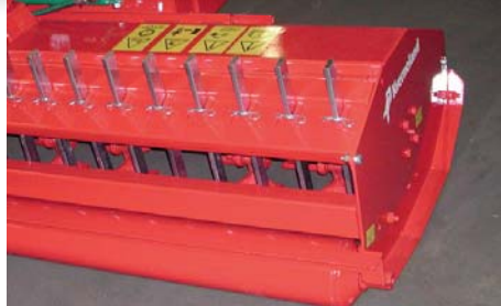
The Kverneland FHS can be equipped with rake tines to improve chopping on prunings.
