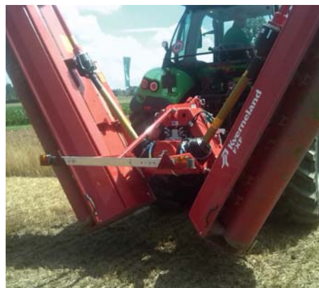
The hydraulic folding main frame is taken from the Kverneland power harrow line; robustness and reliability even in toughest working conditions. The hydraulic locking device is standard.
