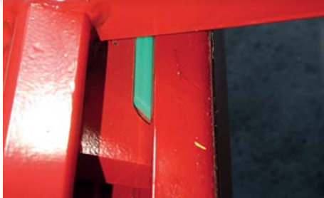
Special nylon plate fitted into sliding guide rail ensures smooth movements without the need for lubrication or maintenance.
