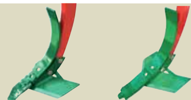
NEW! Quantum share 345mm - always in combination with Knock-on or Tiger carbide point 80mm. It has been designed for use especially against hard soil. The action of the 80mm point combined with the 345mm wing share ensures perfect penetration, and complete flat cutting for a homogeneous weed regrowth.
