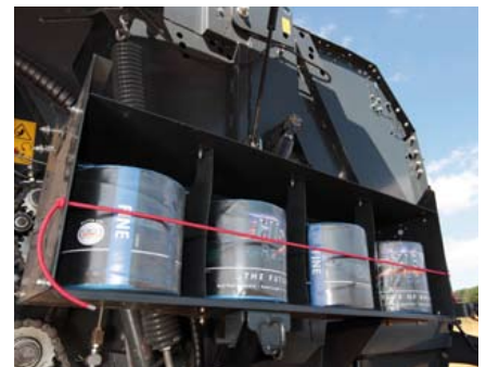
Convenient easy access storage for net and twine for long working days.
