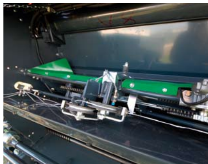
Twin tube fast operating twine binding system.
