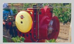
The specially developed fan housing with built-in vertical deflector (model LB 50D) has been designed for the specific requirements in vine spraying and other hedge row crops. It is provided with two adjustable deflectors on top, to guide the air stream.
