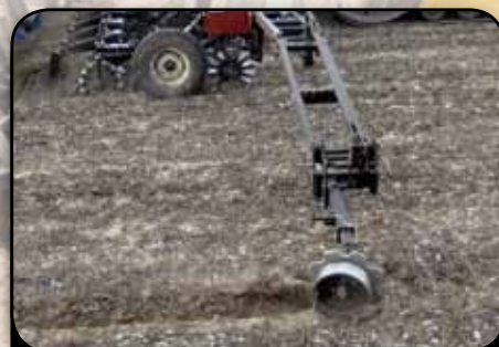
Optional shear-bolt protected row markers with notched blades leave a highly visible mark regardless of soil type or residue level.
