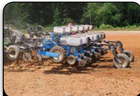
Semi-mounted lift-assist packages that mount directly to 8-, 12- and 16-row planters.
