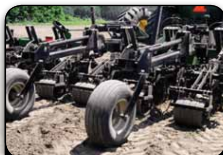
Optional hydraulic lift-assist option for more easily raising the Ripper-Stripper unit.
