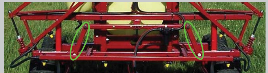
MB spray boom is trapeze mounted to sprayer frame to allow for self stabilizing movement
