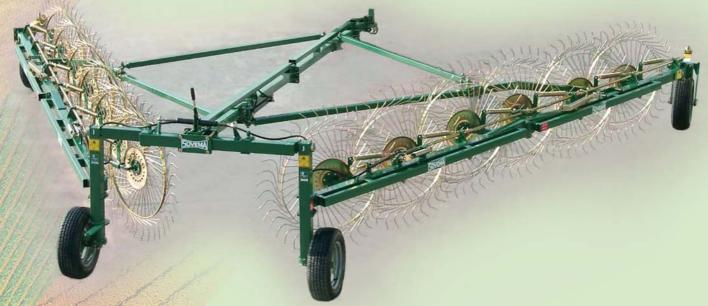
On independent trames, the Sovema pull type finger wheel V-rake is available with 10-12-14 wheels.
