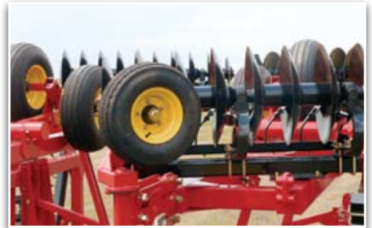
3. Lower the tool to retract wing lift cylinders
