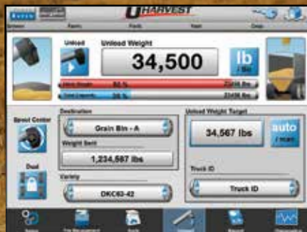
Accu-Save automatically records data for each load and monitors load distribution
