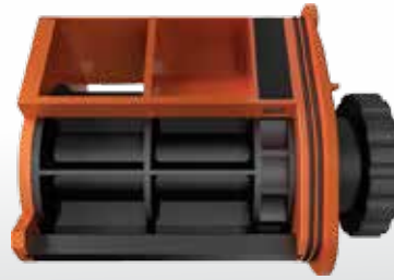
Half-width cartridge for seeds such as flax, lentils and hybrid rice.
