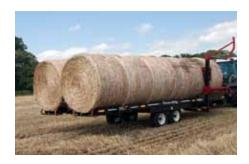
After bales are lifted onto the carrier deck a pusher moves the bales rearward. Powered by two hydraulic motors, the pusher has two settings that are selected on the handheld remote. The operator can choose the most efficient speed and torque for varying conditions: 'high' for dry hay and straw; 'low' provides additional torque for wet or high moisture silage bales, and the pusher moves with less speed.
