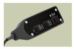
A hand-held control works with the tractor remotes to operate all the functions of the bale carrier. The bale carrier uses two sets of tractor hydraulic outlets.
