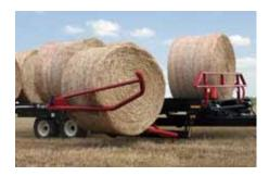
The pickup arm gently lifts the bulk of the weight of the bale and pivots the bale into position before lifting it onto the deck. The pusher, powered by two hydraulic motors, slides the bales rearward on graphite coated carrier beams. To unload, the carrier deck tips back and the bales are pushed off to form neat, tight rows. This entire system means more efficient bale handling, less damage and more bales moved each day.
