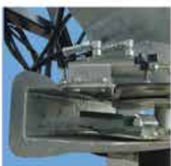
Hydraulic Shut-Off Gate
