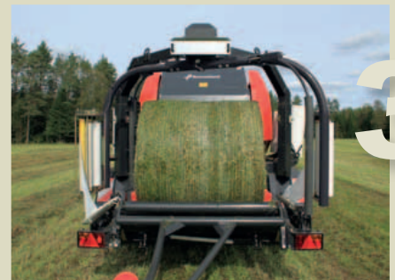
As soon as the bale is transferred away from the baler, the tailgate automatically closes, and baling of the next bale can start.
