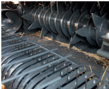
The PowerFeed rotor gives positive intake in all conditions.
