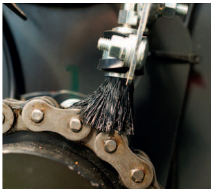
Automatic chain lubrication is standard with lubrication activated continuously at a pre-determined level for each individual chain.
