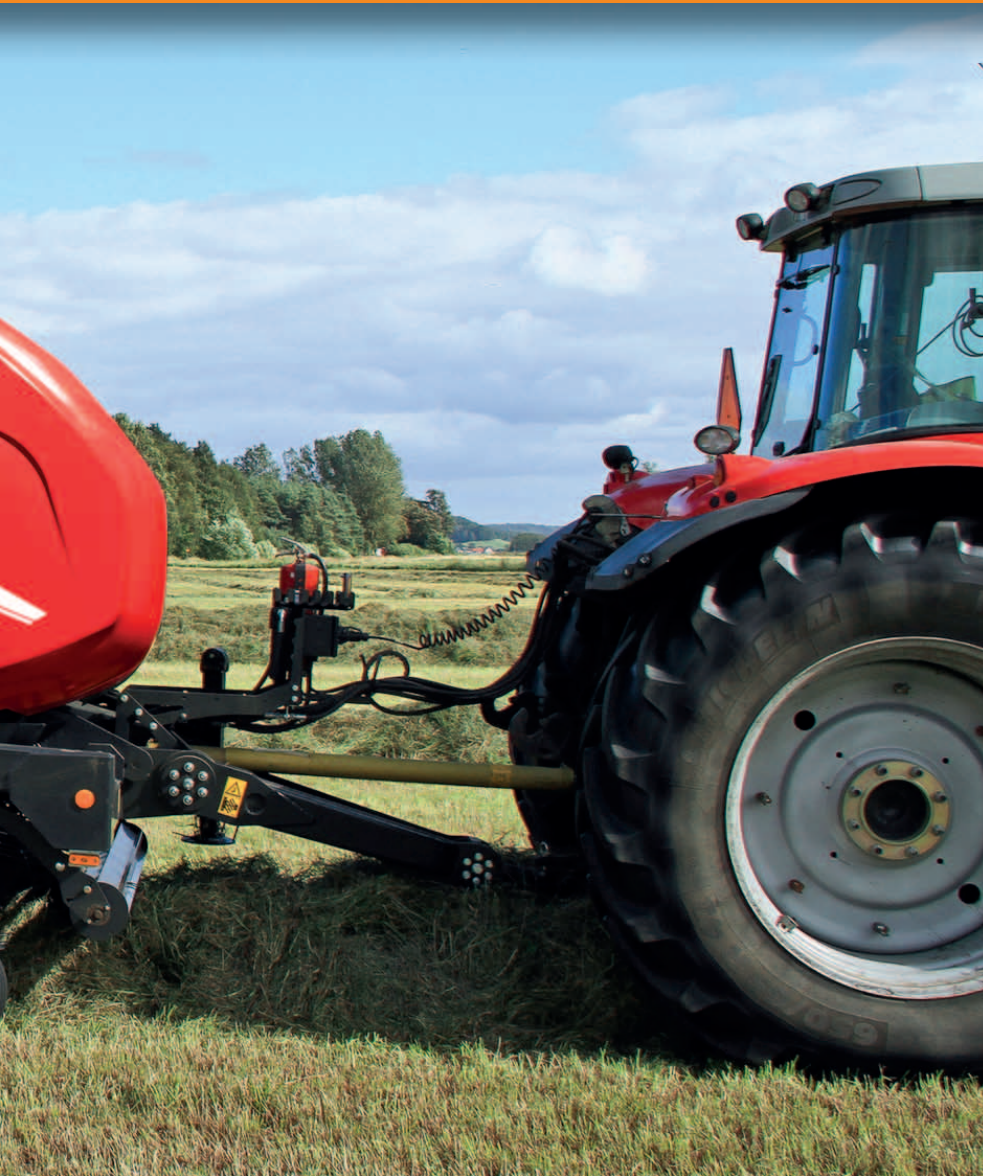
Once the net is applied to the bale the wrapping table is transferred to the tailgate of the baler.
