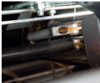
Twin tube fast operating twine binding system.
