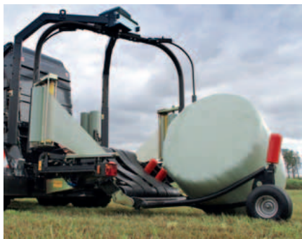
Bale on end kit is available as option. During transport the kit is automatically transferred into a safe position inside the wrapping unit.
