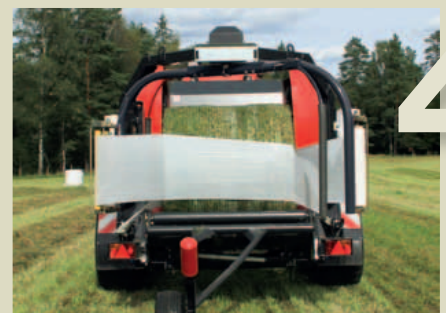
The wrapping table moves very fast to the pre-stretchers and wrapping starts instantly.
