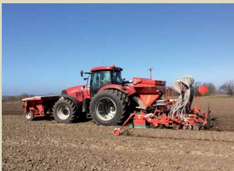
i-drill PRO in combination with DF-1 fronthopper. The DF-1 is for the fertiliser and the hopper of the i-drill PRO for the seeds.
