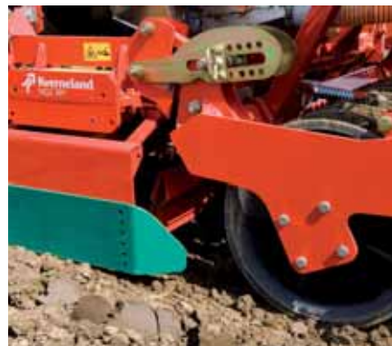
Innovative and precise depth control The packer roller of the power harrow is now mounted on a newly developed parallelogram. The exact seeding depth of the coulters bar running behind the roller frame can be set independently of the working depth and tine wear of the power harrow. The parallelogram can be adjusted in 2.5cm steps, easily and without the need for tools. The adjustment is made on both sides of the power harrow, thus ensuring constant seeding depth.
