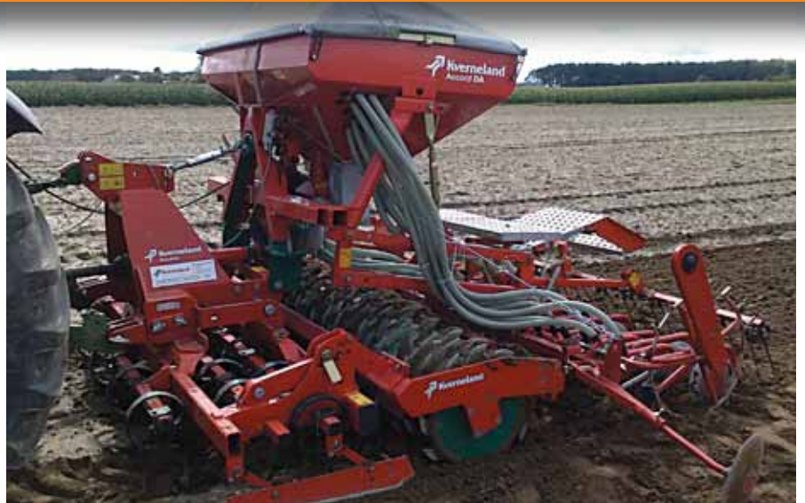
DA, 3m working width, in combination with the Access seedbed cultivator
