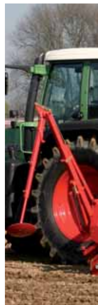
The hydraulically folding track marker with shear-bolt overload protection is mounted directly on the trough of the power harrow.
