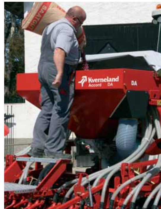
Loading step for safe and secure hopper filling
