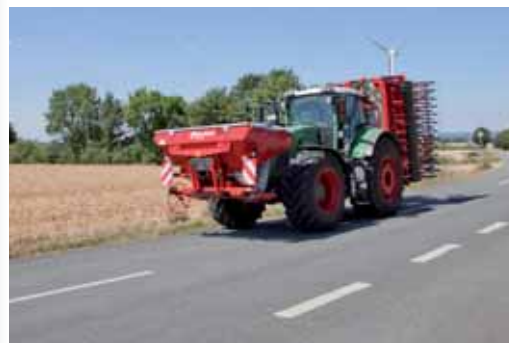
Can be folded to a width of 3.0 m for safe road transport.
