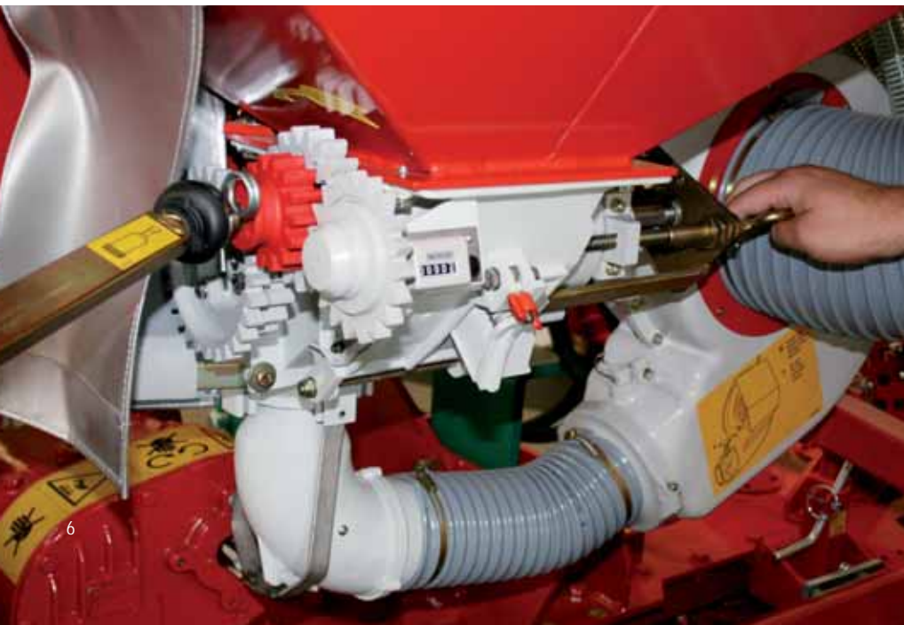
Adjustment of the metering device requires no tools
