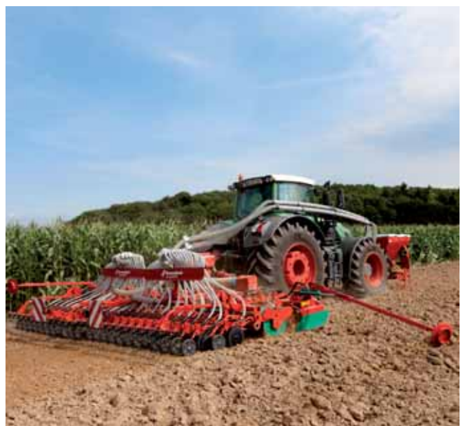
Optimum positioning of the seed delivery hose ensures good seed diffusion.
