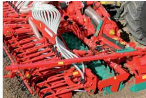
The hydraulically folding track marker with shear-bolt overload protection is mounted directly on the trough of the power harrow.
