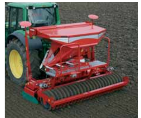
Conversion made simple! In a matter of minutes, the solo machine can be converted into a power harrow/seed drill combination. The coulters bar is attached directly to the roller frame and can quickly and easily be hitched thanks to the readily accessible hydraulic and electronic interface.
