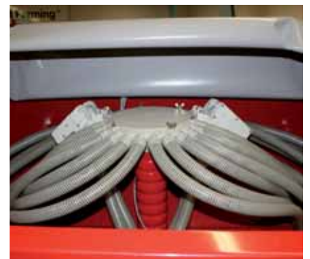
Distribution head inside the hopper
