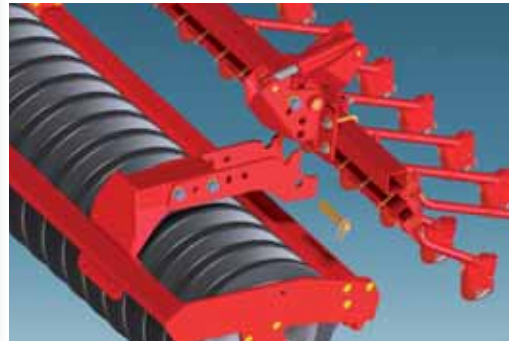
Coulter-bar rapid coupling system (fits all Kverneland rollers)
