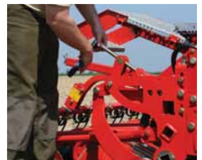
The mechanical coulter pressure adjustment is standard equipment, the hydraulic version is optional
