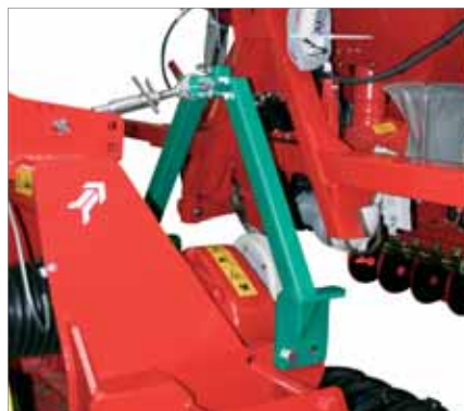
Quick-hitch triangle interface with power harrow
