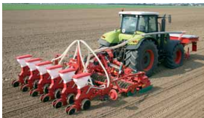
The DF-1 hopper used for fertiliser during precision sowing of up to 8 rows
