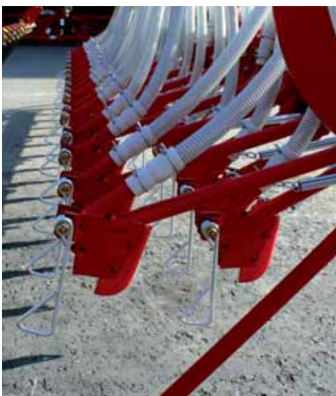
Suffolk coulters with double entry for fertiliser application and seeding in one pass.
