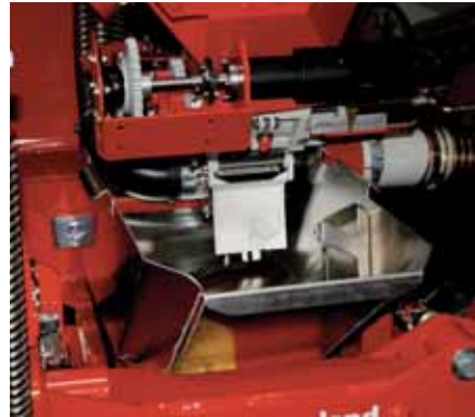
Easy calibration due to patented placement of the metering device.
