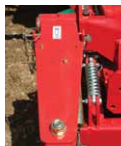
Overload protection of the marker arm
