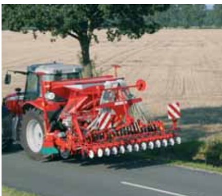
The heavy modules (hopper and power harrow) are positioned directly behind the tractor. This arrangement optimises the position of the centre of gravity, meaning less lifting power is required, and ensures the manoeuvrability of the tractor. Road lights are fitted as standard, ensuring safe road transport at any time of the day or night.
