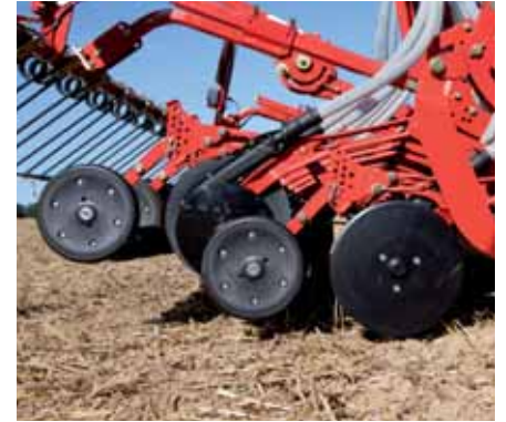
Should the power harrow need to be used solo during sowing, the coulters bar and metering landwheel can be lifted completely via the two integrated hydraulic cylinders of the optional hydraulic coulters bar lift system. This is especially advantageous if furrows are to be closed or if the headland is only to be tilled.
