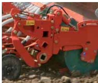
The coulter bar is directly connected to the packer roller frame.
