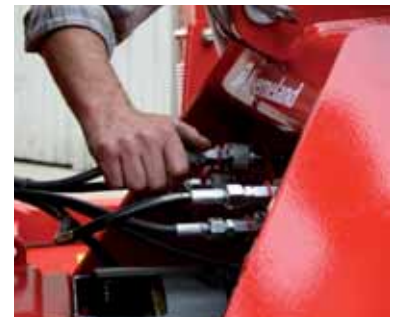
Interface of the hydraulic and electric connections in the headstock of the power harrow
