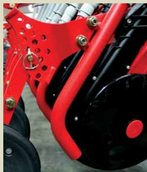
CX-II coulter with double entry for fertiliser application (red tube) and seeding (black tube) in one pass.
