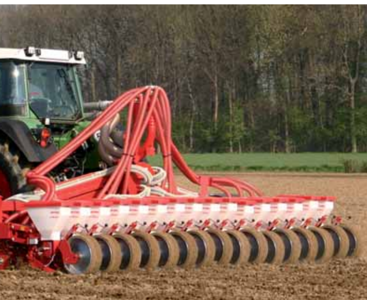
In combination with a precision seed drill, the DF-2 front hopper can be used for row fertilising (up to 16 rows).
