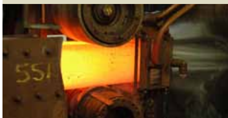
Frame induction heat treatment.
