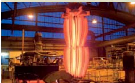
12 hours carburising heat treatment for each mouldboard.
