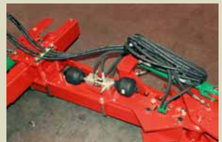
As standard, 2 accumulators are fitted to the BE plough for safe steering
