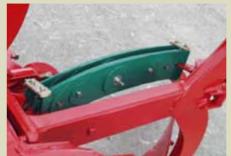
Double spring package - with 14 leaves (1400 kp)
