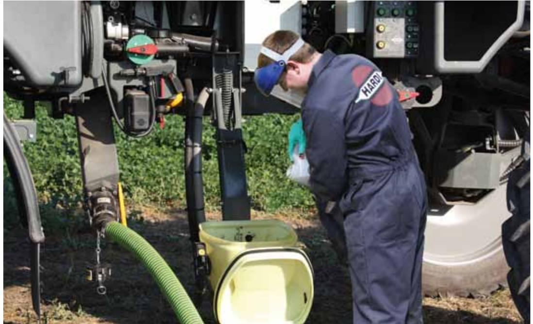
Loading chemicals is safe and easy with the high capacity TurboFiller. Fixed to a parallelogram suspension arm the TurboFiller is lowered into position to provide waist high access to the hopper. The lid has a dust proof seal and the operating controls are positioned on the left side of the TurboFiller.
