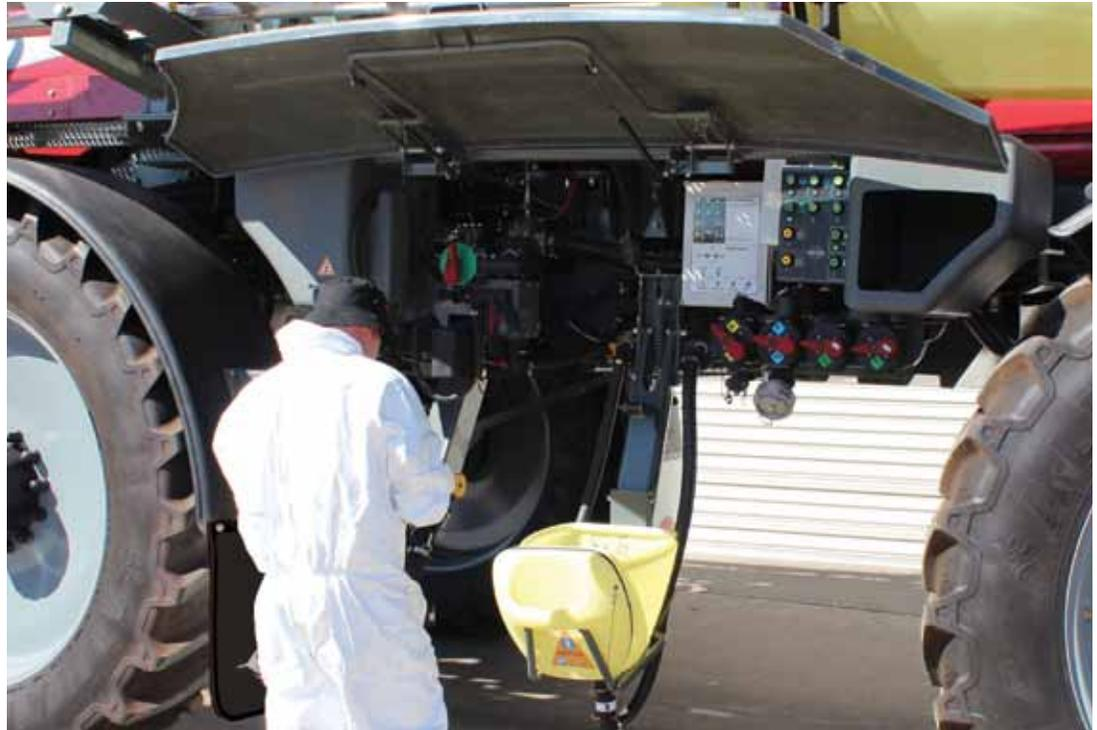
A WorkZone cover, supported by a gas strut, protects the WorkZone and doubles to provide operator protection for when the boom is folded and you are standing under the nozzles.
