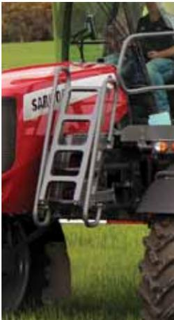
Easy access to the platform and cab is via the front facing heavy duty ladder. It automatically folds up out of the way when the transmission is engaged and folds down when the transmission park is selected.
