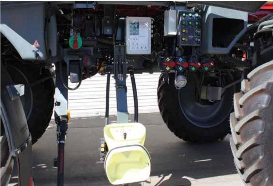
The WorkZone console provides switching for electric motor drive valves that control main or rinse tank, Venturi, pump on/off, tank rinse nozzles, boom nozzle, engine rpm and agitation. An LED identifies which valve is in operation.
