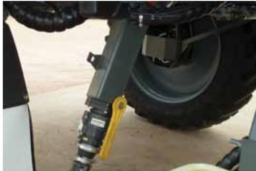
Filtered FastFill or Banjo filtered FastFill valve
