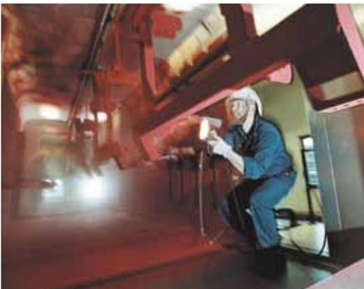
The chassis and all other steel components have received anti-corrosive treatment before the application of a high quality paint finish.
