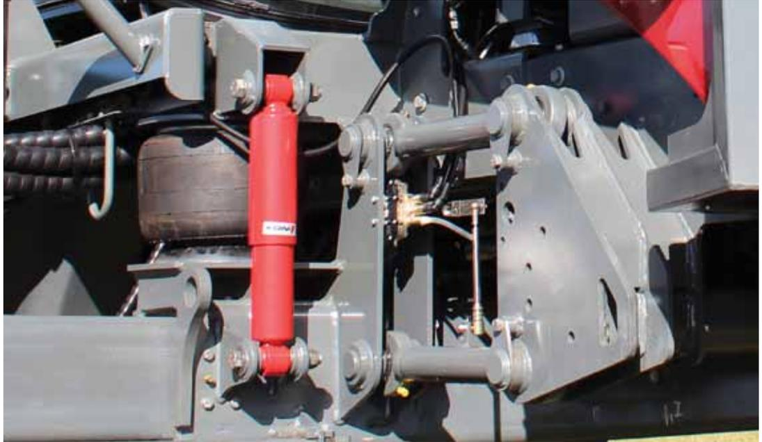
Auto level air ride suspension combined with the flexible high strength chassis delivers an enviable ride for the operator.
