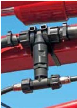
There will still be liquid running through the boom tubes when the distribution valves are closed. A pressure valve in front of the boom sections ensures that the pressure in the sections will be not higher than 10 psi., so the non-drip valves will not open.
