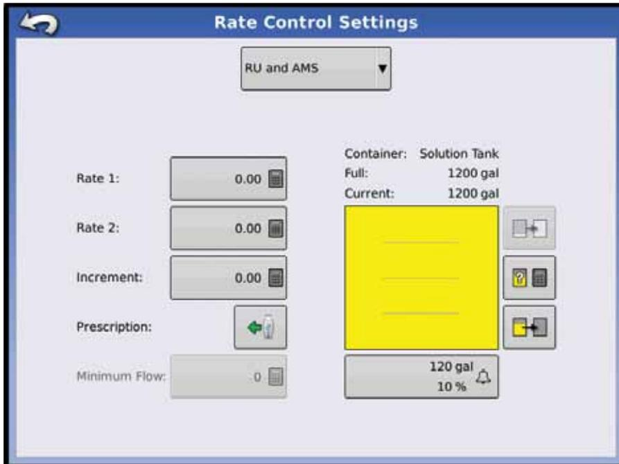
The dosage is set up in the product tab on the main menu. The HC 9500 works as standard with 2 preset dose rates, between this the operator can easily shift by just pressing the button 1 or 2.
