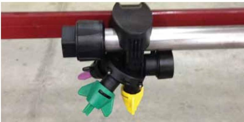
The TERRA FORCE boom is standard equipped with triplet nozzle holders to enable nozzle changes by simply rotating the assembly.
