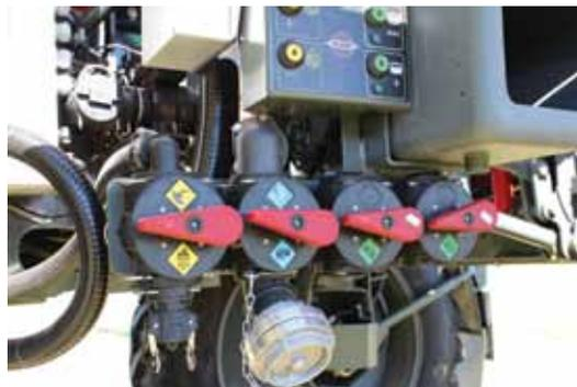
Rinse Tank fill and drain, Main Tank batch fill and drain valves
