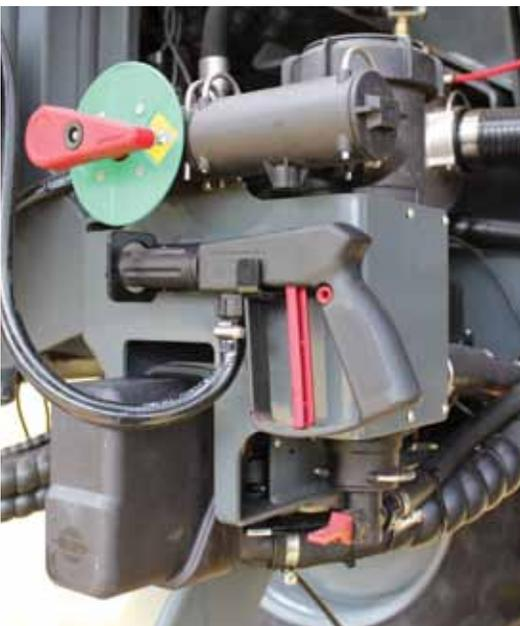
A 60S hand gun run by a flowjet pump connected to the rinse tank is used to clean up around the work zone.
