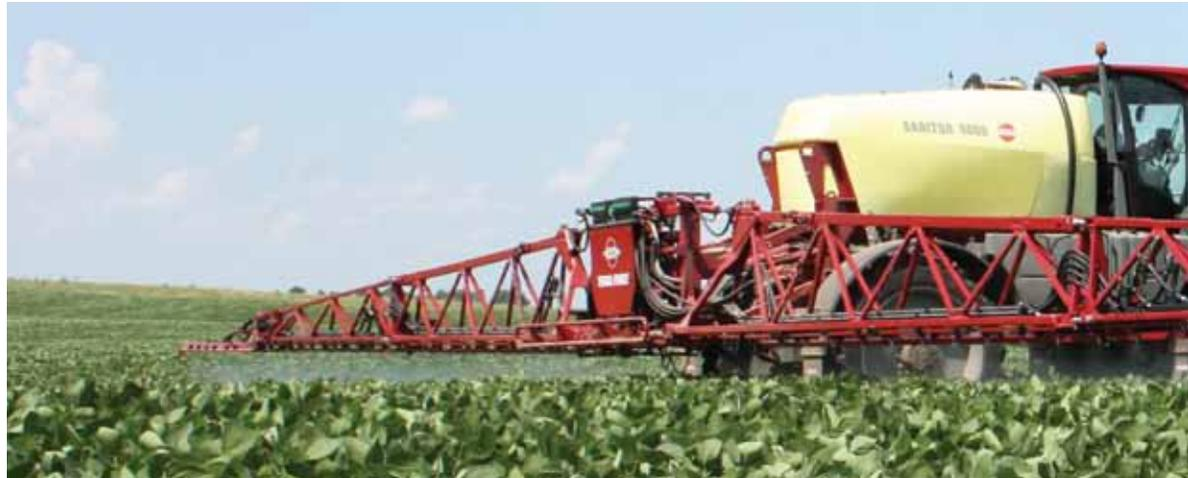
Built strong utilizing heavy duty three dimensional truss construction for high performance and is available in sizes 88, 90, 100, 120 and 132 feet.
