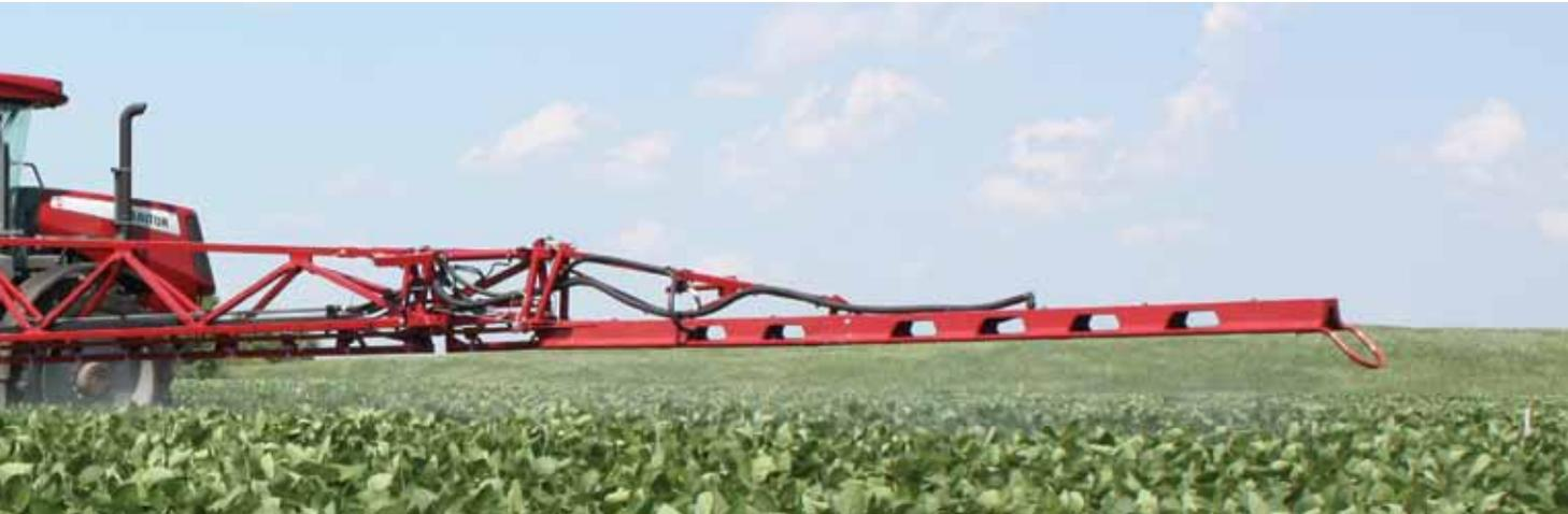
The TERRA FORCE boom is designed to reduce turbulence over and around the nozzle. A continuous mounting rail provides variable nozzle position mounting and easily accommodates 10" nozzle spacing.
