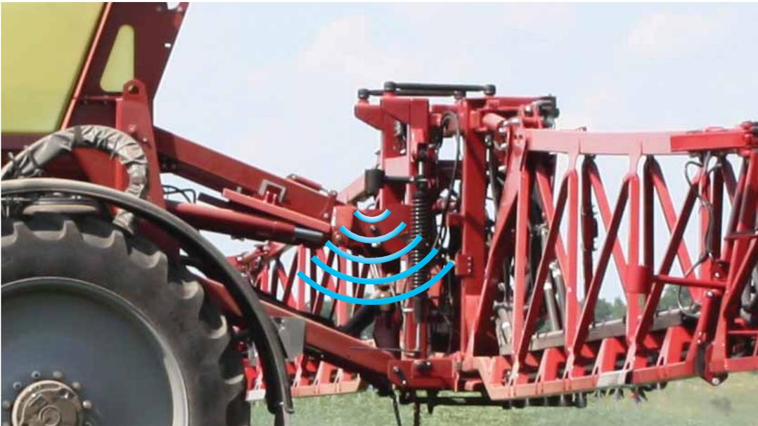
Active roll, sensor, suspension and cylinder
