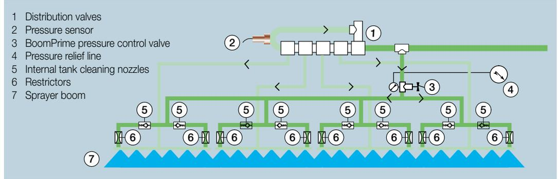
The optional BoomPrime is a low pressure circulation system for HARDI booms. The spray liquid can circulate to the nozzles before the actual spraying starts. It prevents sedimentation and permits flushing of the boom lines without spraying onto the ground.
