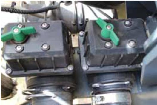
Main tank and rinse tank source valves
