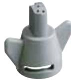
Designed for application of liquid fertilizer. The patented QUINTASTREAM nozzle ensures optimum distribution with overlap. Fertilizer is applied in solid streams, minimizing the risk of phytotoxicity. Five [5] streams of liquid are distributed at different angles and flows. Highest flow is from the middle stream and lowest in the outer overlapping streams. Boom height 14-40 inches, however this system tolerates boom and ground undulations without affecting the quality of distribution.
