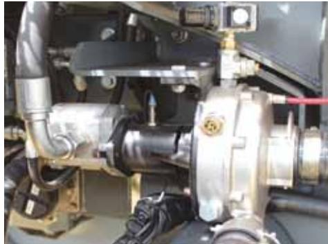
The SARITOR DynamicFluid4 fluid system is driven by a high performance Run-Dry centrifugal pump capable of up to 170 gpm and a operating pressure range up to 160 psi. (see chart below)
