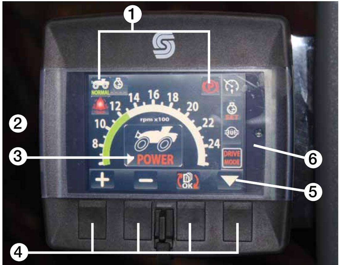
A High resolution multi-functional display terminal for both control of operation of engine, transmission and operator selected control choices. System can be set for metric or imperial display.
