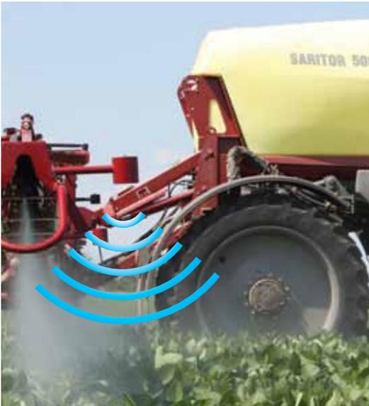
Ultrasonic sensor monitor wing height
