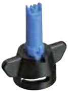
INJET air inclusion nozzles are used for drift management when spraying in sub-optimal conditions cannot be avoided. They have a venturi air inlet between the pre-orifice and the outlet orifice. Very large and slow moving droplets are produced with air inclusion. This makes them less sensitive to wind reducing drift by up to 75% over Standard Fat Fan nozzles.
