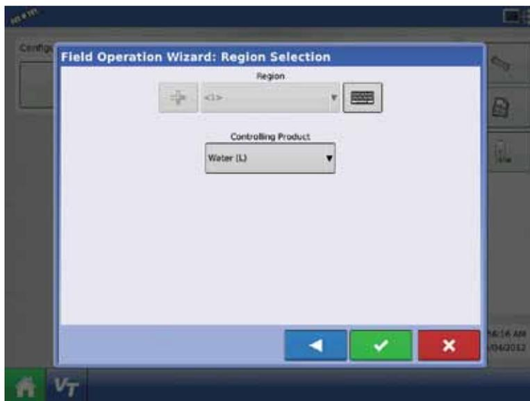
4 Now press the green box with check mark, and the spray job is loaded into the data base, and the run screen view is now available. The grid sign on the bottom task bar, when selected, will bring up the work screen.
