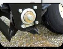
1-bolt flange bearing with 1¾" shaft for durability
