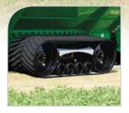
Tracks equalize to follow altering terrain – each track independently cambers to follow ground contours for optimum flotation and minimum compaction
