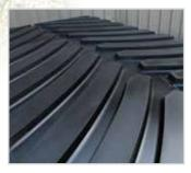
Exclusive belt design with shallow tread belt pattern for greater flotation and traction
