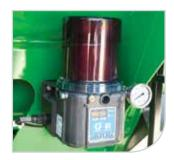
Auto-greaser system for automatic application at more frequent intervals for consistent lubrication of track undercarriage
