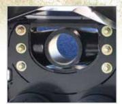
Patent-pending pivot allowing bi-directional rotation of the track for better contact with the ground on uneven terrain
