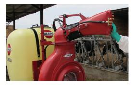
Angling and rotating the cannon from one side to another is easily done. No tools are needed to adjust the spout.
