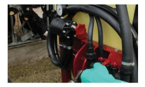
Applying the precise dose is easily chosen by the manifold valves and pressure regulator
