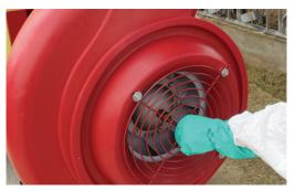
When mixing spray liquid or in transport, the turbine fan can simply be disconnected.
