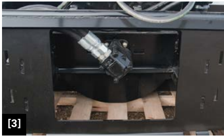
[1] Hydraulic motor chain drive. [2] Wiring harness fits most skid steer brands. [3] A hydraulic motor mounts directly on the fan and auger shaft eliminating couplers and chain drive assembly.
