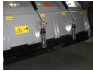
Rear hydraulic protection/grader hood to level the output material.
