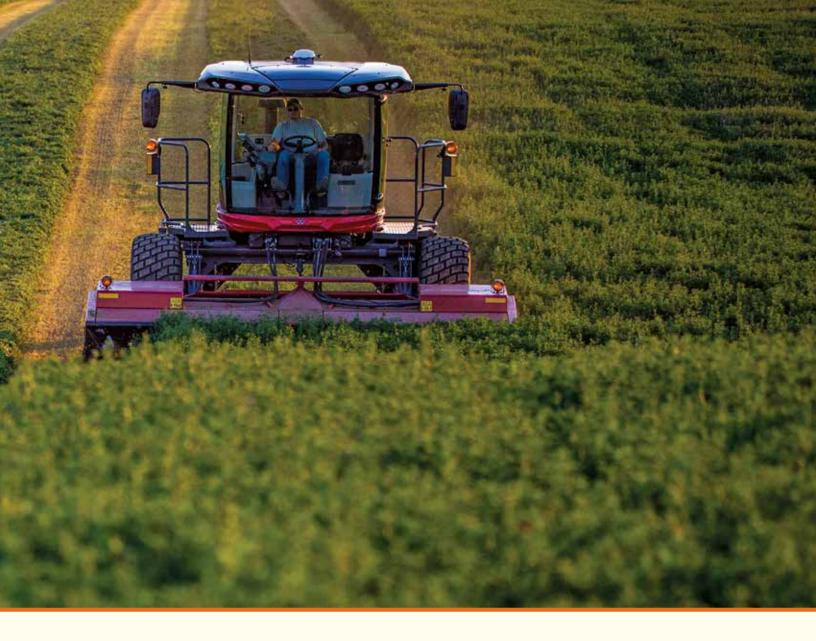
New lighting package features eight front-mounted and two rearmounted lights, providing operators with greater visibility in low-light conditions. LED lights are also optional for even greater visibility.
