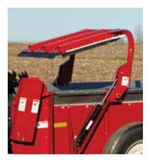
The tight-sealing hydraulic endgate provides peace-of-mind when hauling high-moisture loads that could leak onto roadways or into the farmyard. Optional on the SP3710.
