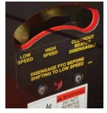
Two-speed apron drive is standard equipment on most models except the SP3735 & SP3748. These two models come standard with the Electric-overhydraulic variable speed drive.
