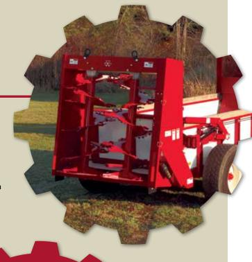
Beater gearboxes on the vertical beater assembly are mounted at the top of the assembly rather than the bottom, to avoid damage.
