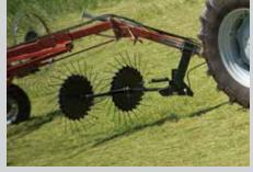
AN OPTIONAL CENTER KICKER WHEEL is available on both 3900 Series wheel rakes, as well as all 1500 Series rakes to turn the entire windrow and eliminate any wet spots beneath unraked crop.
