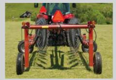
**FOLDED FOR TRANSPORT,** the 3986 and 3983 models fold to 8 feet — all without ever leaving the tractor seat.
