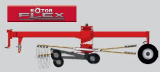
**THE ROTORFLEX SUSPENSION** features "jet-effect" lifting and lowering, which means the front lifts first and lowers last, to keep tines from diving into the ground.
