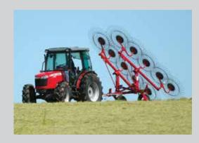
**ONE SINGLE-ACTING CYLINDER** folds both wings for easy transport.
