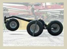
Our dual rotor models feature "jet effect" rotor lifting. When lowering the rotor from headland to working position, the rear end of the rotor touches down first (like on an airplane). This prevents the tines from scalping the ground and contaminating the windrow. It also extends tine life.
