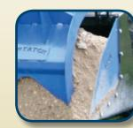
optional bolt-on side plates for finer material handling
