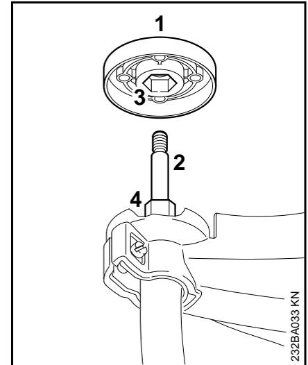
The thrust plate (1) is shipped with the DuroCut 5-2 and PolyCut 6-3. It is only required for these mowing heads.
