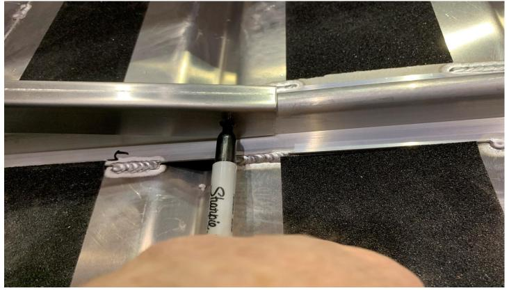
2. Remove mounting crossmembers, you should have 8 marker dots to use as drill pattern. Drill ribs from both sides. 8 holes in total(careful not to drill bottom of boat).
