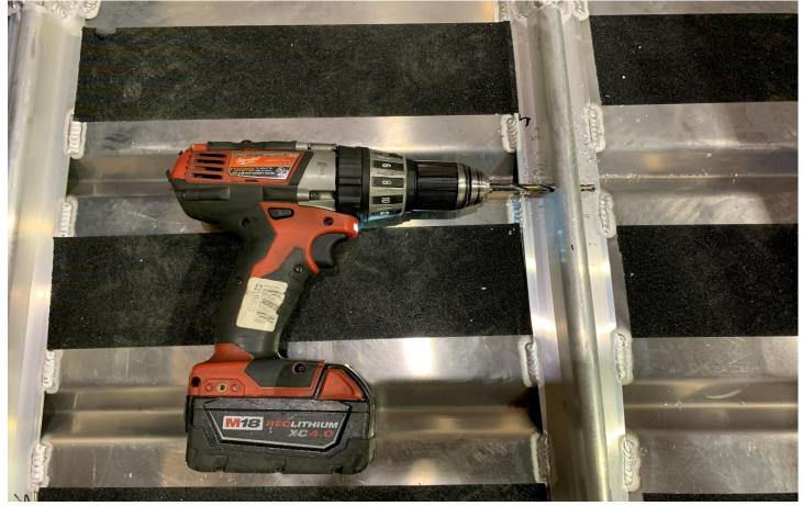
Finish by running the drill thru both holes. This will help align the holes.
